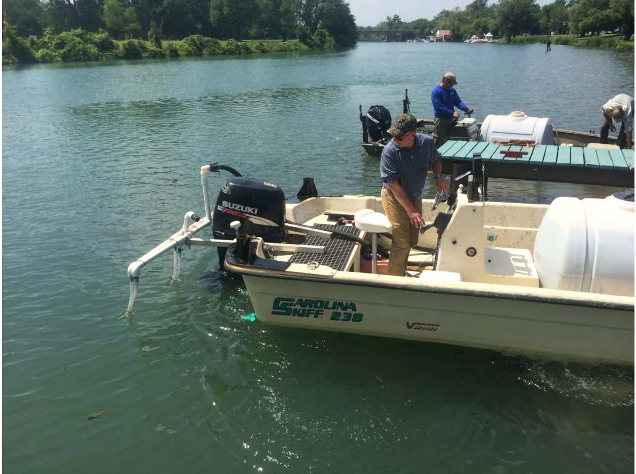
Photo A-3 Application skiff set-up.
